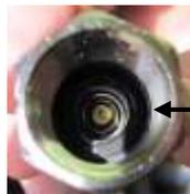
The washer fits into this part of the Quick Connect and should sit flush against the top to ensure a good seal.
